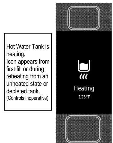
Above-Screen Three-HWD Status Screen
